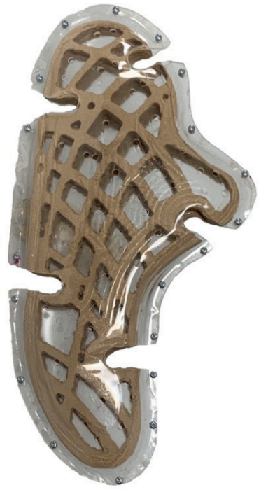
Wood structure framework(MDF)
